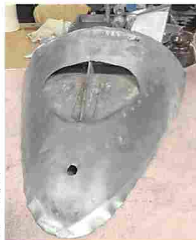
F-86 canopy fairing after corrosion treatment
