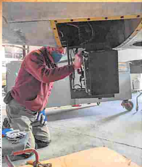
Danny prepares the transponder for installation in the F-86
