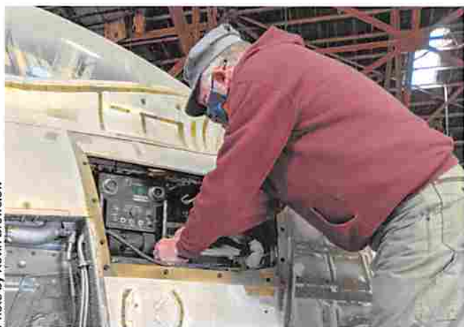
Danny installs the AN/ARC-27
